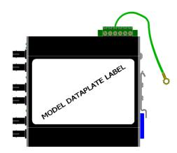
Both V- legs of the power input connector are connected to chassis internally on the PCB. Connecting a drain wire (shown in green) to earth ground from one of the V- terminal plugs as shown here will ground the switch and the chassis. The power leads from the power source should be limited to 3 meters or less in length.
